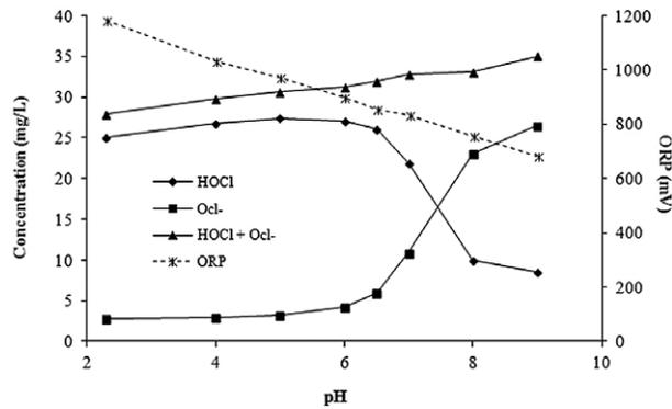
**FIG. 2.** CONCENTRATION OF HOCl, OCl<sup>-</sup>, THEIR SUM AND OXIDATION REDUCTION POTENTIAL IN ACIDIC ELECTROLYZED WATER (AEW) OBTAINED BY ELECTROLYSIS OF 1.25 G/L NaCl AQUEOUS SOLUTION AND ADJUSTED TO INCREASING pH
