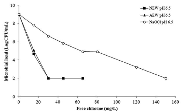
**FIG. 3.** MICROBIAL LOAD OF *PSEUDOMONAS FLUORESCENS* AS A FUNCTION OF FREE CHLORINE CONCENTRATION OF NEUTRAL (NEW) AND ACIDIC (AEW) ELECTROLYZED WATER SOLUTION AT pH ADJUSTED TO 6.5
